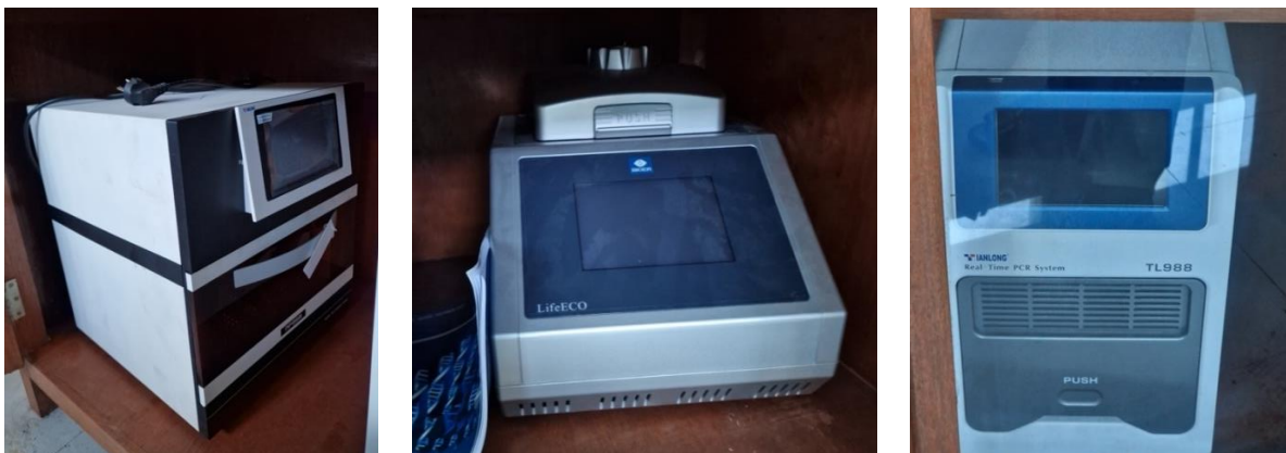
Figure 5: Some machines present at NIA and currently not in use: nucleic acid extraction system (left); thermocycler (center); and real-time Polymerase Chain Reaction (PCR) machine (right).
