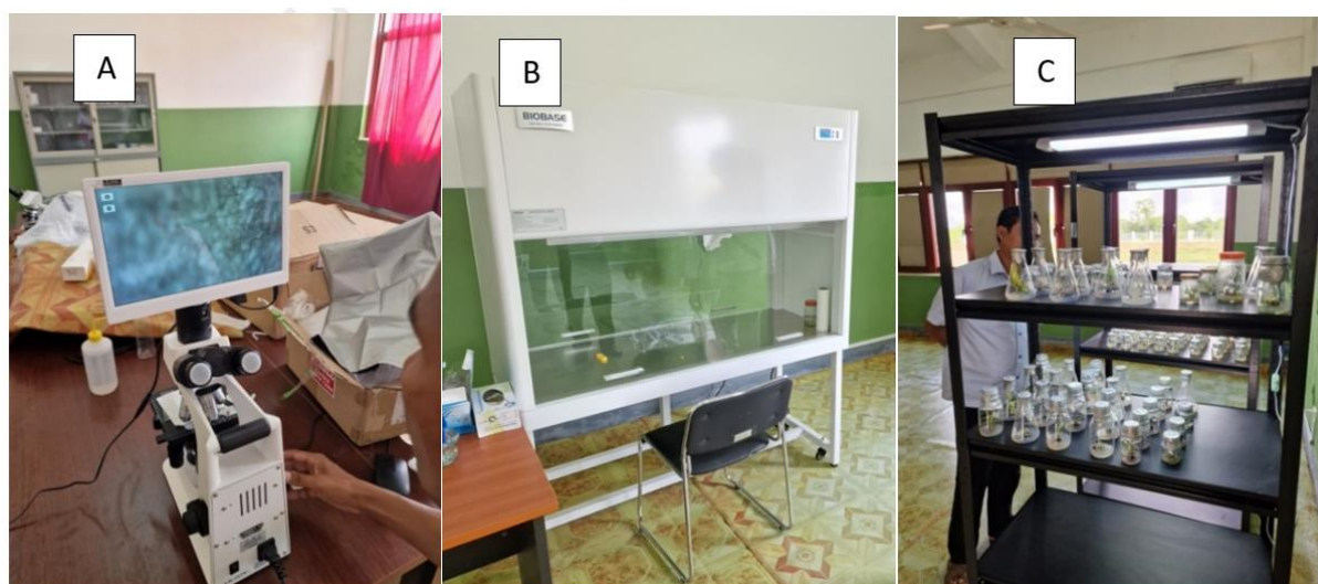
Figure 10: Light microscope with direct imaging (A); air flow bench for working in sterile conditions (B) and various cultures of hydroponic baby plants (C).
