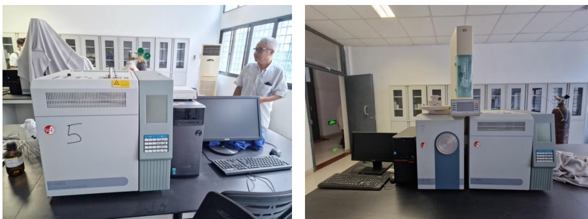
Figure 2: Gas chromatography GC 400A with its nitrogen tank (left) and Gas chromatography mass spectrometer with the its helium tank (right) at NIA.
