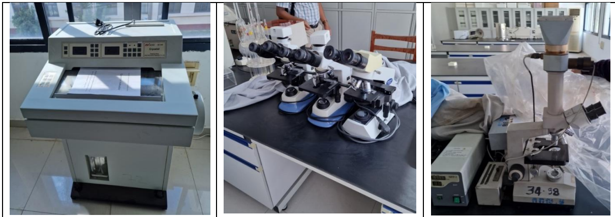
Figure 4: Freezing microtome (cryostat, left), light microscopes (center) and inverted microscope (right) at NIA
